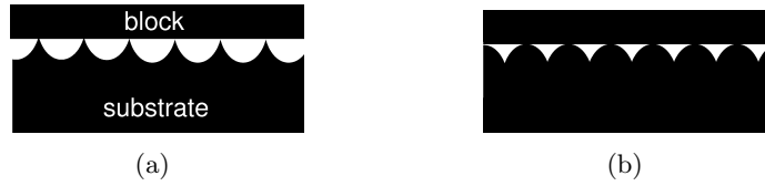
Abbildung 4.19: The figure shows the contact between a rigid block with a flat surface and a rigid substrate with periodic surface structure. The two substrate surfaces in (a) and (b) have the same surface roughness power spectrum. Note that the empty volume between the surfaces is much larger in case (a) than in case (b), and therefore one would expect the leak rate to be largest.
