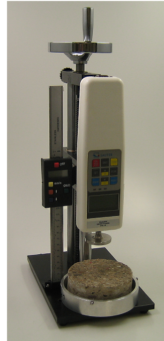
Abbildung 3.5: Picture of the instrument produced by SAUTER GmbH (Albstadt, Germany) used in the experiment. A rubber block is squeezed against different surface samples. The displacement s of the upper surface of the rubber block is changed in steps while the restoring force F is measured by a force cell.
