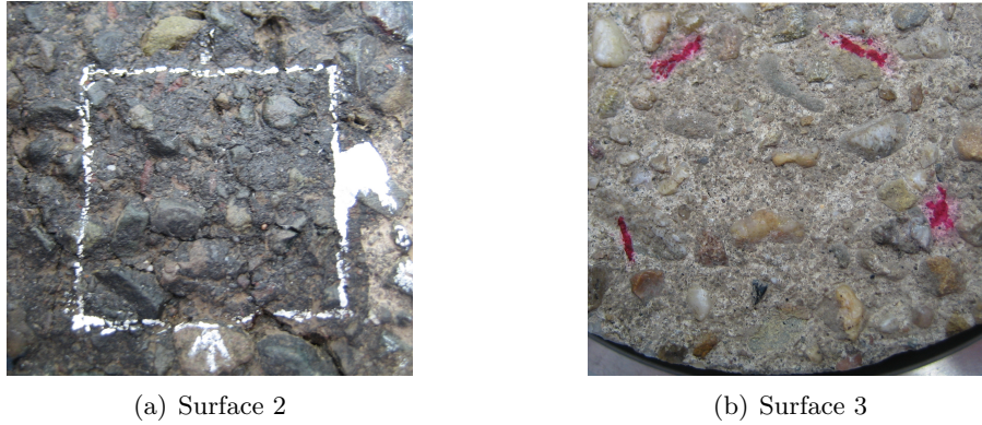
Abbildung 3.9: Pictures of two surfaces used for the experimental investigation. (a) An asphalt road surface, denoted as surface 2. (b) A concrete road surface denoted as surface 3.
