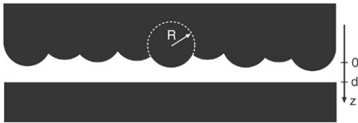
Fig. 7. Contact between rough surface and a plane. All asperities with height z greater than the separation d make contact.
