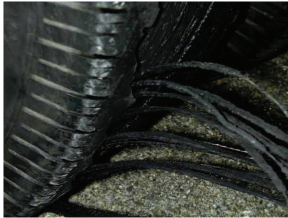
Figure 1. Catastrophic crack propagation in rubber, resulting in an exploded tyre.
