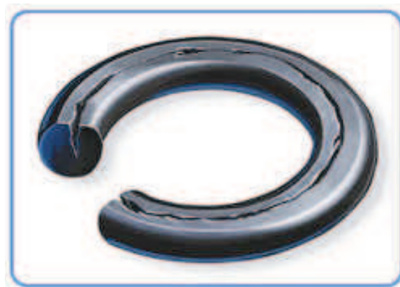
Figure 2. A crack in an over-compressed rubber O-ring.
