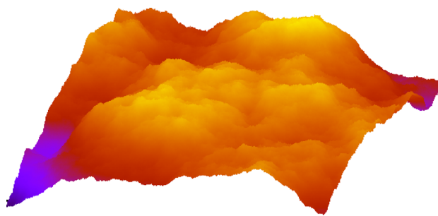
Fig. 9 Topography picture of a surface produced by the eroding process described in Fig. 8 after removing 76,290 layers of blocks. The surface plane consists of 2,048 \times 2,048 blocks. The surface is self-affine fractal with the Hurst exponent H = 1 (or fractal dimension D_f = 2 ) (see Fig. 10). The width of the removed particles (or blocks) is a = 0.1 \mu\text{m} . The surface has the rms roughness h_{\text{rms}} = 2.1 \mu\text{m} and the rms slope \kappa = 1.04
