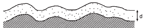
FIG. 5. The adhesion interaction pulls the elastic slab into complete contact with the rough substrate surface.
